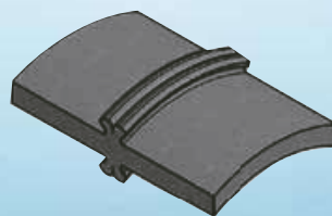
Non Perfectly Connected Bead
