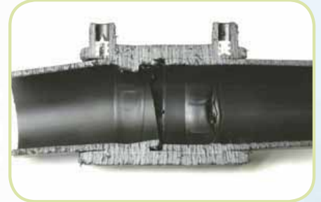
Off-Centering of the Pipe on the Left Side and Wrong Welding Parameters Setting
