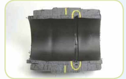
Wrong Centering of the Pipes
