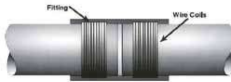
Typical Electro fusion Joint
