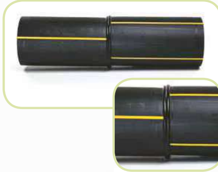
Off-Centering of the Pipe on the Left Side
